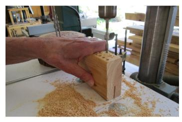
1. Here he uses a drilling machine to drill cavities for the bees in a 2x4 piece—something that is probably more commonly found around your house! He drills holes into the narrow side so the cavities for the bees to next in can be as deep as possible. Try not to make your holes too shallow—the bees will get cold!
